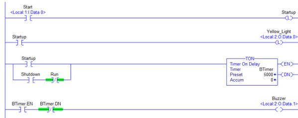
This can be prevented by adding additional logic to rung “0”:
