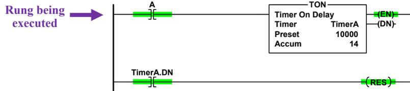
The next time the **TON's** rung is executed (after the **TON** was reset):
