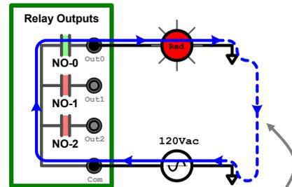
Note that, when multiple nodes are “grounded” within a circuit, they are considered to be connected to a “common ground” that provides a path for current to flow between any of the grounded nodes. The conductive paths between the commonly-grounded nodes are typically not shown in the figures.
