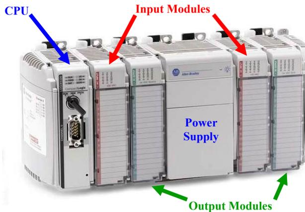
Shown above is a modular Allen Bradley CompactLogix PLC that contains:
