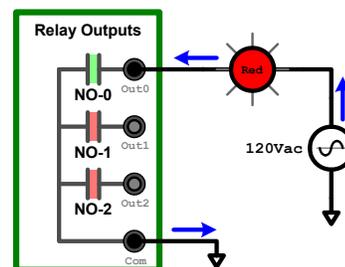
Sinking outputs allow for the simultaneous control of various loads that utilize different supply voltages provided that the different voltage sources can all be connected to a common ground.
