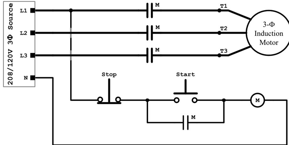
Schematic Diagram of the Basic Start/Stop 3 $\Phi$  Motor Controller
