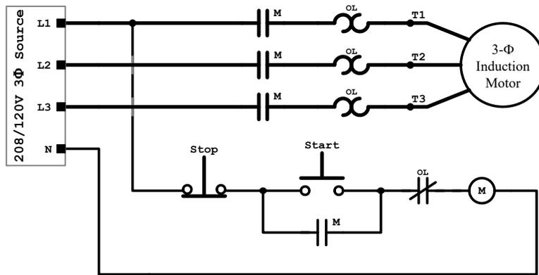
Due to their location in the circuit, the OL heaters are often mistakenly assumed to de-energize the motor when an overload occurs.
