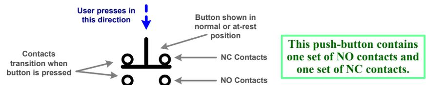
Note that the combination push-button is typically designed such that one type of contacts will transition slightly faster than the other type when the button actuated.
