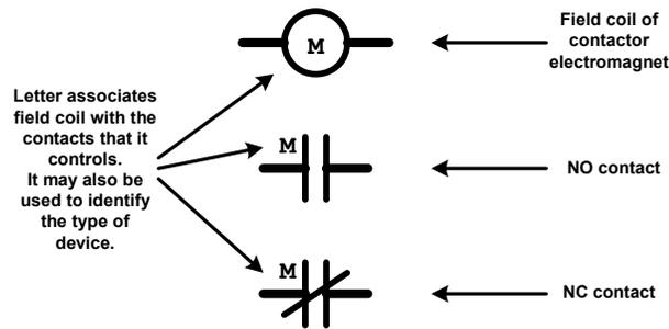
Although the same symbol is utilized for both the main contacts and the auxiliary contact, the auxiliary contact (along with any other control-circuit component) is typically drawn in a lighter type-face compared to that utilized for the main contacts (and any other power-circuit components).
