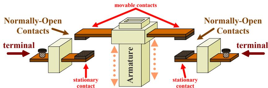
(The contacts are **actuated closed** by energizing the electromagnet's field coil.)
