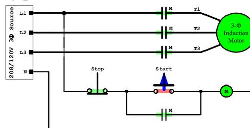
When used for this purpose, the auxiliary contact is often referred to as a **“hold-in contact”**.
