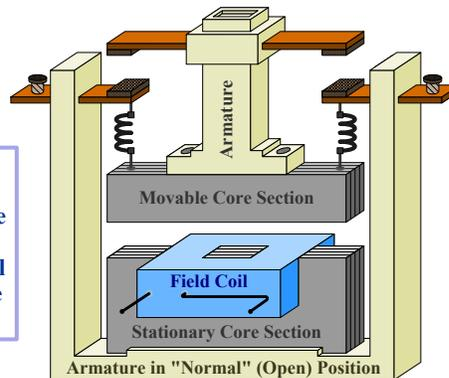
This figure only depicts one set of the NO main contacts that would be placed in-series with one of the lines that supply power to the load. A three-phase contactor would have two more sets of contacts attached to the armature.
