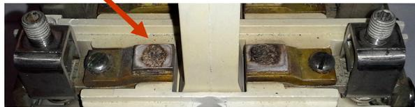
If the damage becomes excessive, the contacts must be replaced in order to prevent a contactor failure and/or operational problems with the contactor's load.
