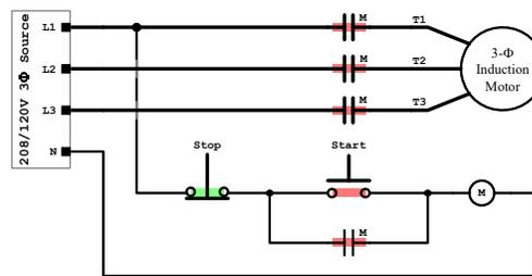
Note that, even though a █ may appear behind a contact or pushbutton, the actual flow of current also depends on whether or not the other devices in the circuit allow for a closed-loop path for current flow.
