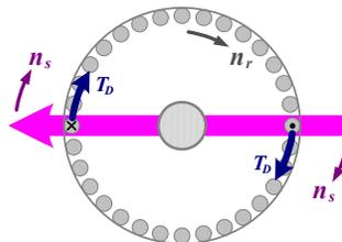
The operation of the rotor is a function of both the **torque,  $T_D$ ,** **developed** by the motor, and any external forces experienced by the machine’s rotor that oppose its rotation.
