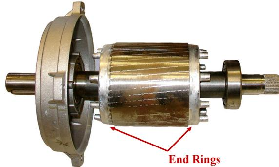
The ends of the **conductive bars** are **shorted** together by a pair of **conductive rings**, forming the “Squirrel-Cage” aspect of the rotor while, more importantly, providing the **closed-loop paths** that are required for current flow within the rotor conductors.
