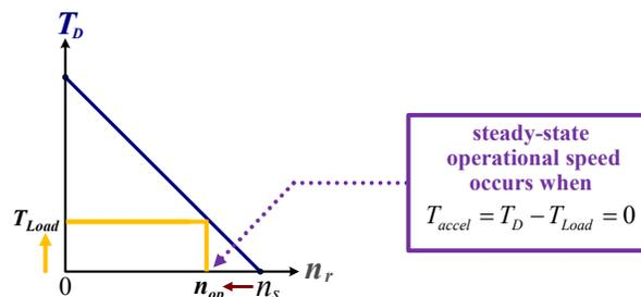
If a **load torque** is applied to the rotor **after** it reaches synchronous speed (no-load conditions), then the rotor will **slow down** to a new **operational speed** ( $n_r = n_{op}$ ) at which the **developed torque**,  $T_D$ , is equal to the **load torque**,  $T_{Load}$ , and  $T_{accel} = 0$ .
