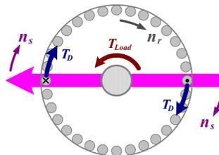
The **acceleration torque**,  $T_{accel}$ , experienced by the rotor is the difference between the amount of torque ( $T_D$ ) available to accelerate the rotor and any coupled mechanical load ( $T_{Load}$ ), as defined by:
