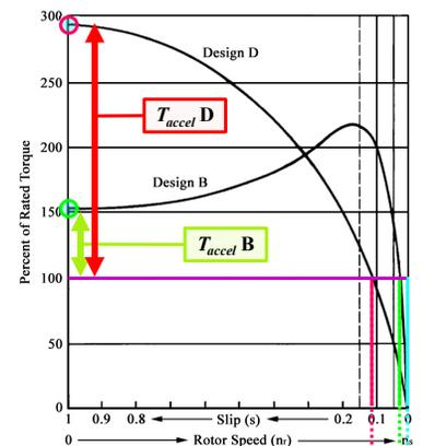
As often occurs, there is a trade-off when switching to a **Design D** motor for the increased “starting torque”, and that trade-off is poor speed regulation. In comparison to a **Design B**, changes in load torque result in a much greater variation of the rotational speed for a **Design D** motor.
