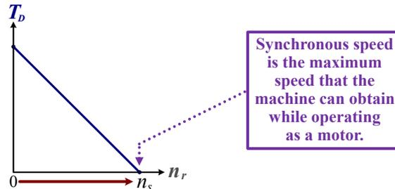
Note that, once the motor reaches **synchronous speed**, it develops no torque because the field lines no longer cut through the rotor conductors (i.e. – they're synchronized). Due to this limiting effect, **an induction motor cannot accelerate beyond synchronous speed** by its own power.
