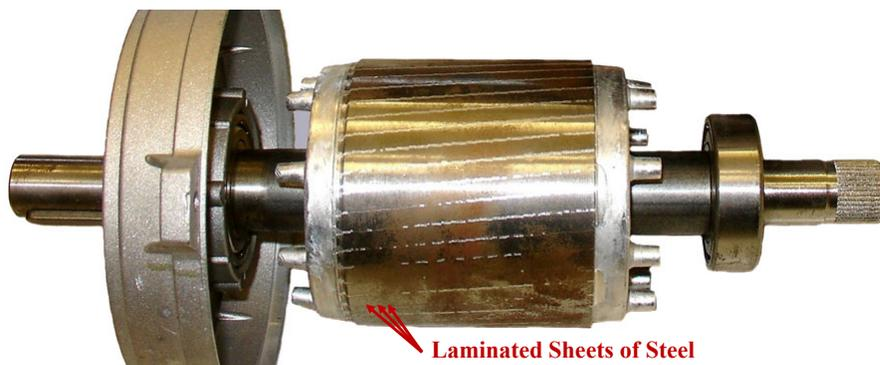
The **laminations** provide insulation between the sheets that form the rotor, thus preventing currents from flowing length-wise through the rotor unless they travel within the embedded bars.
