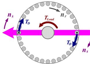
The **total load torque**,  $T_{Load}$ , experienced by the machine's rotor is the total torque, applied to its shaft, that opposes rotation.
