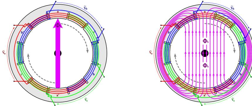
And it is **rotational speed** of the constant magnitude, directionally-rotating stator field,  $\Phi_s$ , that fundamentally governs the overall operation of the Squirrel-Cage Induction Motor.
