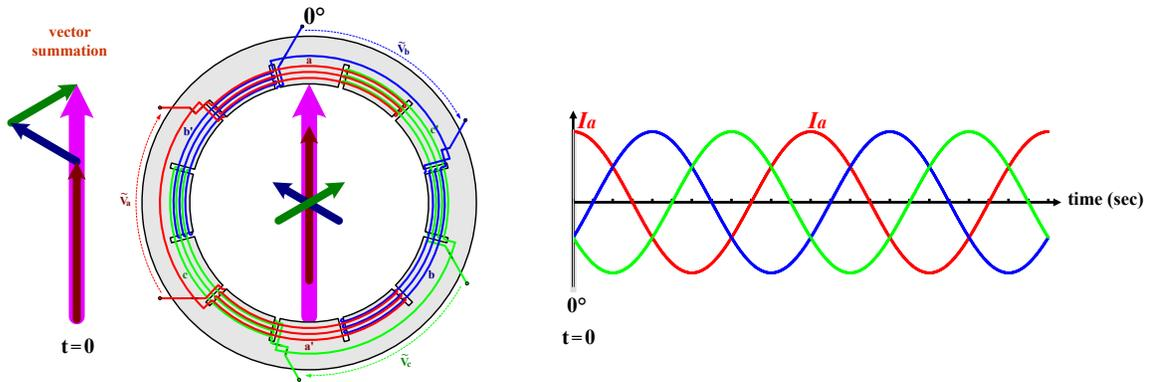
The net stator field induced within the rotor region by the currents flowing in the stator windings is the **vector sum** of the three individual magnetic fields.
