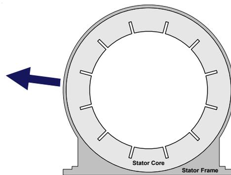
The **stator** consists of a **frame**, a **core**, and a set of **windings**.
