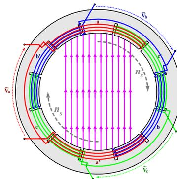
At any point in time, the net stator field induced by the set of three, symmetrically-placed, stator windings, passes through the rotor region from one side to the other in an (ideally) linear manner.
