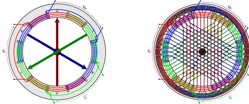
Since the **windings** are placed symmetrically around the stator, the fields created by each of the windings are oriented such that they pass through the rotor region at angles that differ by  $120^\circ$ .
