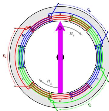
The **synchronous speed**,  $n_s$ , of an induction motor is defined to be the **rotational speed** of the **stator field**.
