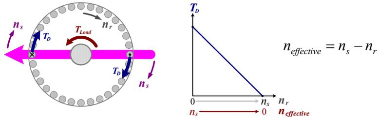
Since the **developed torque,  $T_D$** , is **proportional** to the **effective speed,  $n_{effective}$** , the developed torque will decrease linearly as the rotor speed increases, eventually decreasing to zero as the rotor reaches synchronous speed.
