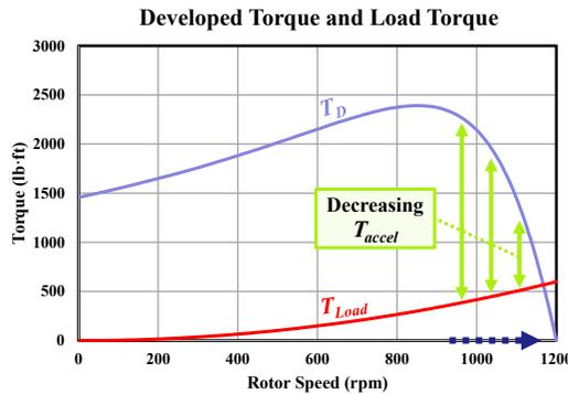
Although the rate of acceleration has decreased, the rotor speed still continues to increase as long as  $T_{accel} > 0$ .
