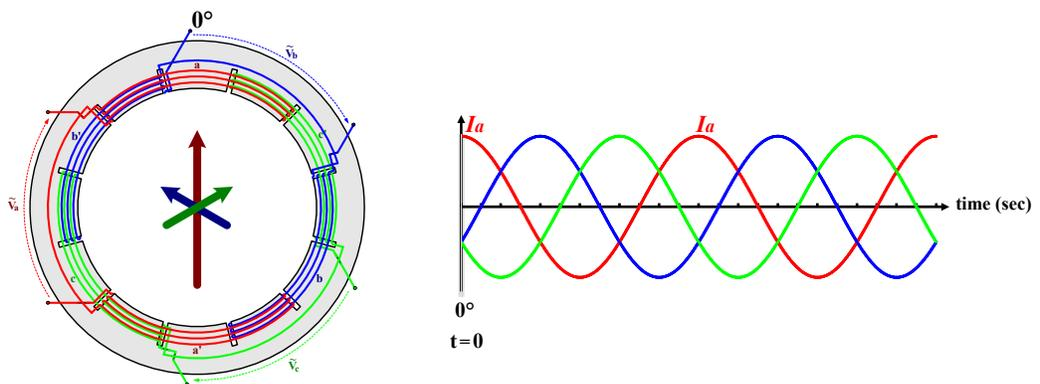
Furthermore, since the windings are supplied with a balanced set of 3Φ currents that differ in phase by  $120^\circ$ , the magnitudes of the individual **fields** created by the windings also vary sinusoidally and differ in phase by  $120^\circ$ .
