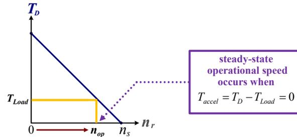
Similarly, if a **load torque** is applied to the rotor at “**startup**”, then the rotor will only be able **accelerate** up to the **speed**,  $n_{op}$ , at which the **developed torque**,  $T_D$ , equals the **load torque**,  $T_{Load}$ , and  $T_{accel} = 0$ .
