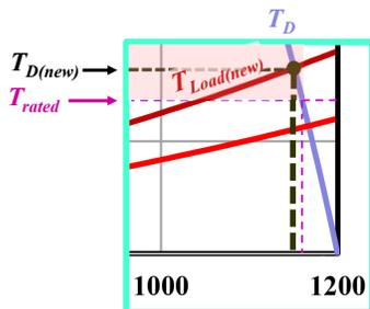
Whenever  $T_D$  is greater than rated torque, **the motor will draw larger-than-rated currents** that, if allowed to flow for an **extended amount of time**, will cause the **motor to overheat**.
