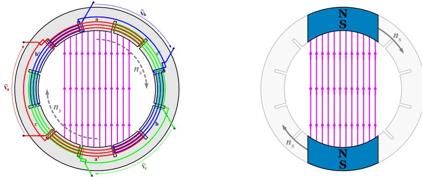
It is a “**two-pole**” construction because the resultant field within the rotor region is similar to the field that would be created by the opposing poles (one N & one S) of two permanent magnets placed on opposite sides of the stator.
