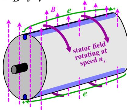
The **polarities** of the voltages are opposite due to the direction that field lines cut through each of the conductors.
