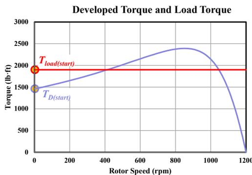
If the motor fails to start, the large starting currents that the motor normally draws will quickly **overheat the motor** unless overload protection is provided.
