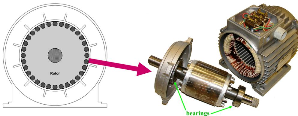
The **rotor** consists of a cylindrical structure that is mounted axially on a central shaft, the ends of which are held in place by a set of bearings that allow the entire structure to rotate freely when placed within hollow center of the stator core.
