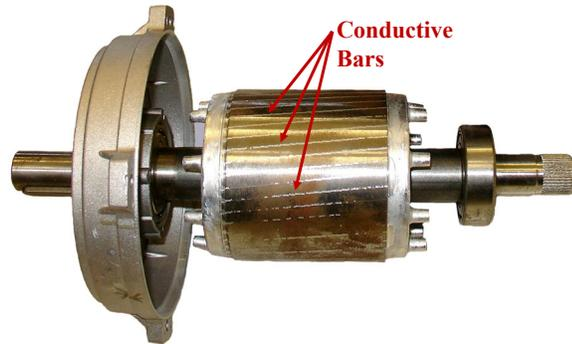
A “Squirrel-Cage” rotor is constructed using laminated sheets of steel, through which holes are cut in order to provide openings that span the entire length of the rotor, within which a set of **conductive bars** are embedded.
