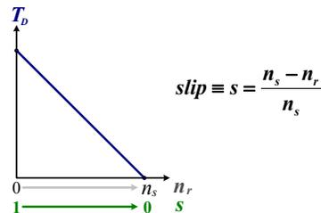
As **rotor speed,  $n_r$** , increases linearly from **0  $\rightarrow$   $n_s$**  (synchronous speed), **slip,  $s$** , decreases linearly from **1  $\rightarrow$  0**.
