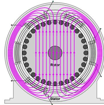
Although the stator and the rotor are electrically isolated from each other, their operation is linked together by means of a mutually-linked **magnetic field** that passes through both regions.
