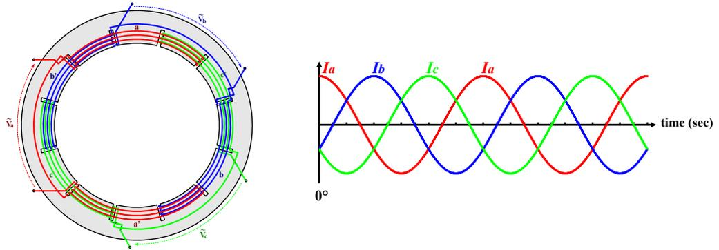
The **stator** contains **three stator windings**, each of which are split into two halves. The half-windings are placed symmetrically around the interior of the stator core, and then wired together to form either a **Y** or  $\Delta$  load for a 3 $\Phi$  source.
