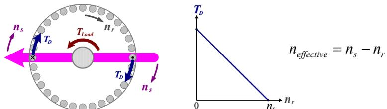
Thus, based on the previous analysis, the **torque-speed curve** shown above defines the operational characteristics of an “**ideal**” induction motor for rotor speeds ranging from  $0 \rightarrow n_s$ .
