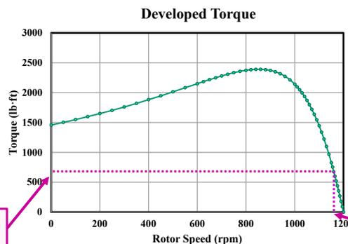
Also note that a rated speed of 1160 rpm relates to a slip of 3.33%.
