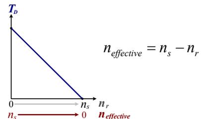
**Effective speed**, which is the difference between the rotational speeds of the stator field and the rotor:
