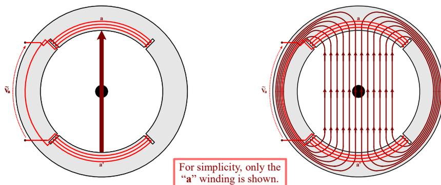
When **current** flows through a winding, the winding creates a **magnetic field** that is proportional in magnitude to the current and has closed-loop field lines that pass through "rotor region" and back around through the outer portion of the stator.
