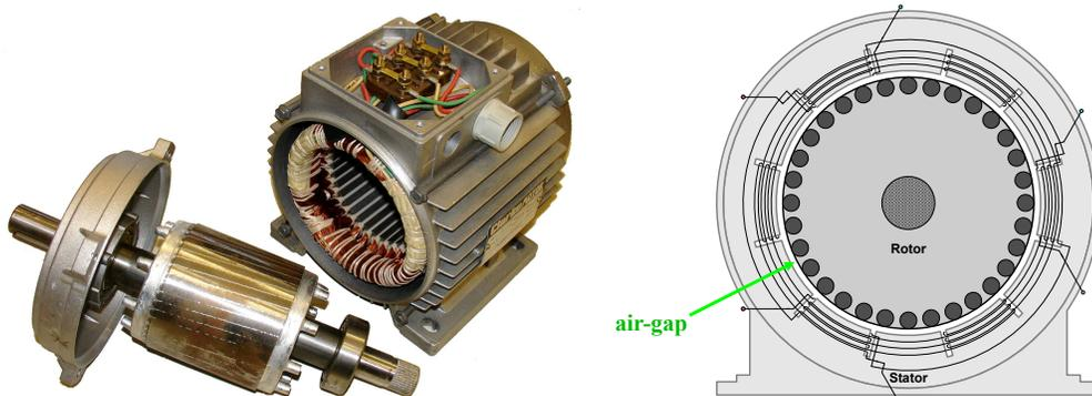
A 3 $\Phi$  Induction Machine has two primary components:
