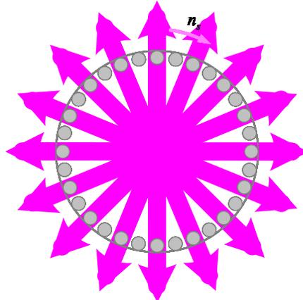
As the stator field rotates within the rotor region, its **field lines** cut across the conductors that are embedded under the surface of the cylindrical rotor.
