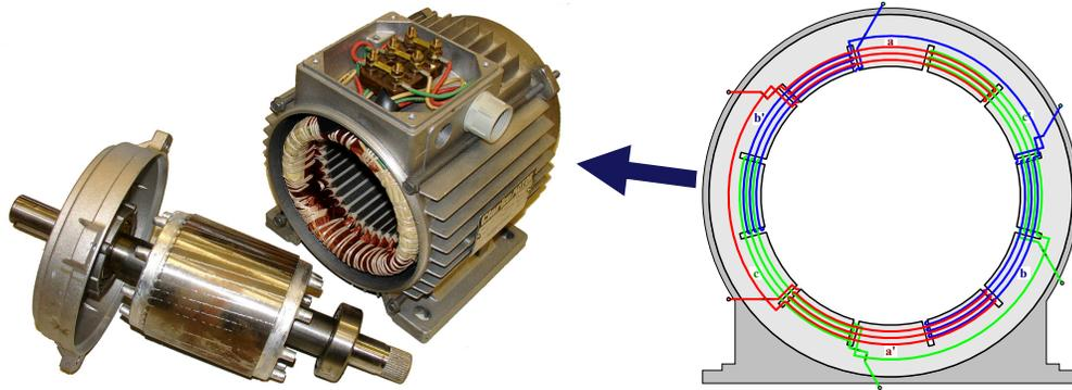
A set of **stator windings** are placed within the slots that are cut into the core, forming an overall magnetic circuit that, when energized, produces the **primary magnetic field** that links with the rotor in order to develop a torque upon the rotor and induce rotation.
