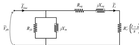
Note that this model does not account for the motor's mechanical losses.
