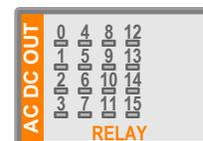
The LEDs on the physical input and output modules can be invaluable when troubleshooting the operation of a PLC-based motor controller. For example, if this system does not start-up when **Start** is pressed, this could be due to either an electrical problem or a logic (programming) problem.
