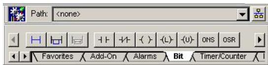
25. Choose the **Bit** tab in the *New Component* toolbar. The **Bit** tab displays instructions that are associated with a single-bit in memory.
