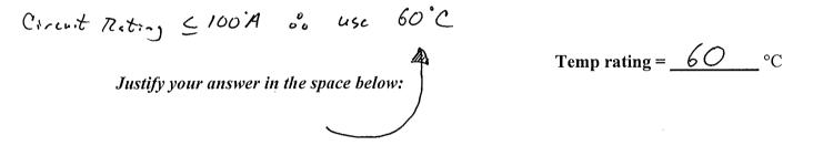
c) Specify the smallest-size, THHN, <u>copper</u> conductors that can be utilized for this feeder assuming that the circuit is composed of three, individual conductors that are run through a separate <u>steel conduit</u>, and that the ambient temperature is 30°C.
