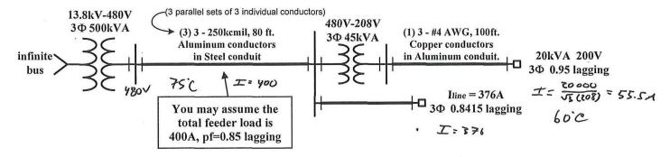
Neglecting any transformer <u>losses</u>, determine the **operational line-voltage** seen at the 20kVA load outlet assuming that rated voltage is present at the secondary terminals of the 500kVA transformer, that the load supplied by the #4 AWG, 100' branch circuit is drawing rated power, and that the total current supplied by the 80' long feeder circuit is 400A at a pf = 0.85 lagging.
