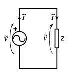
Based on this definition, the impedance Z can be defined in terms of the voltage and current as:
