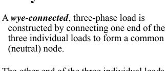
The other end of the three individual loads provide the terminals for connection into a  $3\Phi$  system.
