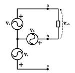
Note – if the neutral terminal is not available, then only *line voltages* can be received from the supply, but <u>not phase voltages</u>.
