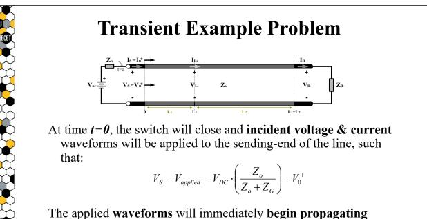
The applied **waveforms** will immediately **begin propagating towards the receiving end** of the line.
