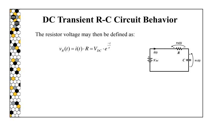
Thus, for a DC voltage source connected to a series resistor-capacitor pair by means of a switch that closes at time t=0:
