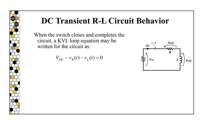
The resistor's voltage, as per Ohm's Law, can be defined in terms of the resistor's current as:
