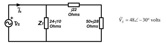
Determine the real power  $P_1$  that is consumed only by the impedance labeled  $Z_1$  in the circuit.
