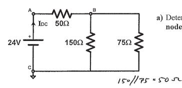
a) Determine the source current I<sub>DC</sub> and the individual node voltages  $V_A$ ,  $V_B$ , and  $V_C$ .
