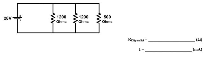
Problem #7) Given your results from Problem #6, determine the magnitude of the current that will flow in the 500 ohm resistor using the Current Divider Rule.
