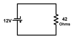
consumed by the resistor in the following circuit. Additionally, draw an arrow labeled with a capital "**I**" to show the direction of current flow in the circuit.
