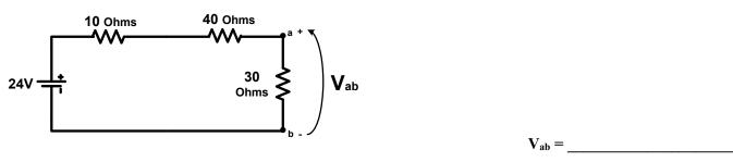
Problem #3) Determine the voltage  $V_{ab}$  as shown in the following circuit using Kirchhoff's Voltage Law.
