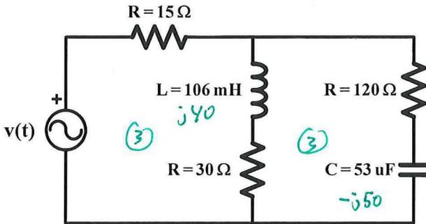
I.e. – express the loads in terms of their impedance values and then perform series and/or parallel conversions to simplify all of the loads down to a single equivalent impedance.
