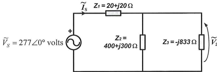
$$\textcircled{6} \quad \left( \begin{aligned} Z_2 \parallel Z_3 &= \left( \frac{1}{400 + j300} + \frac{1}{-j833} \right)^{-1} = (0.0016)^{-1} = 625 \Omega \\ Z_{eq} &= Z_1 + Z_2 \parallel Z_3 = (20 + j20) + (625) = 645 + j20 \end{aligned} \right)$$
