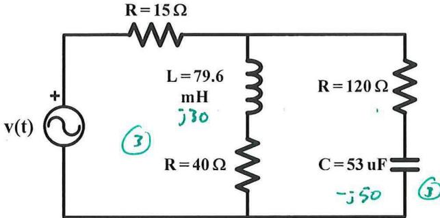
I.e. – express the loads in terms of their impedance values and then perform series and/or parallel conversions to simplify all of the loads down to a single equivalent impedance.
