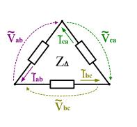
Given a 480V,  $3\Phi$ , Y-connected, positive-sequence, balanced source that is supplying a  $\Delta$ -connected, balanced load with individual phase impedances
