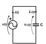
Since the power waveform has a zero-average value, the capacitor consumes zero real power:
