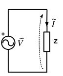
Note that **power factor** is often specified as having a **leading** or **lagging** characteristic, which is based on the angle relationship between the phasor voltage and the phasor current
