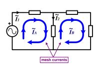
Although the mesh currents are theoretical currents, the <u>actual currents</u> that flow in the various branches of the circuit can easily be determined from the mesh currents, in-turn allowing for solution of any of the circuit voltages.
