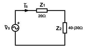
$$\widetilde{V}_{S} = 120 \angle 0^{\circ} \text{ volts}$$
