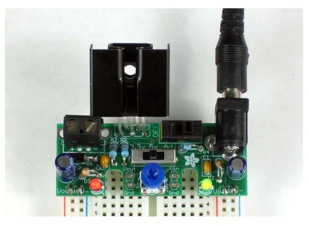
This project details the design of a very low dropout adjustable power supply. A good power supply is essential to electronic projects. While there are many existing designs for adjustable power supplies, this one makes improvements that make it more useful for hobby designs.
