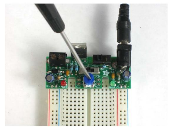
Once you set the pot, the output voltage is not dependent on the input voltage. That is, if you dial in 6V and you switch from a 9V to 12V supply, the output will stay at 6V.
