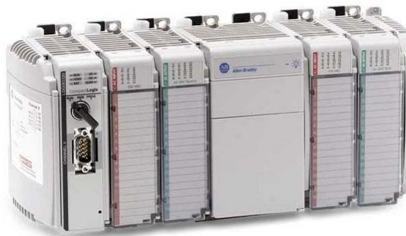
**Shown above is a modular Allen Bradley CompactLogix PLC that contains: a CPU, a 12-port input module, a 16-port output module, a power supply, a 16-port input module, and another 16-port output module.**
