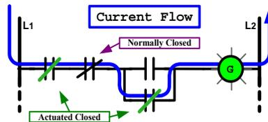
Note that two or more loads may be connected in parallel on one rung when their operation is based on the same conditional logic.
