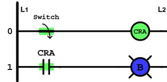
**But, when the switch on rung-0 closes, CRA’s field coil will be energized, in-turn actuating CRA’s NO contact on rung-1.**
