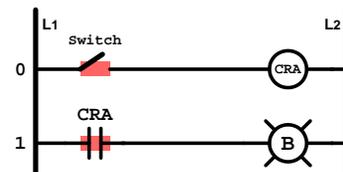
If the switch on rung-0 is initially open, CRA’s field coil will be de-energized, and CRA’s NO contact on rung-1 will be in its “normal” position (i.e. – open).
