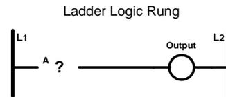
For example: a relay has a spare NO contact available, but a NC contact is needed to implement the required logic.
