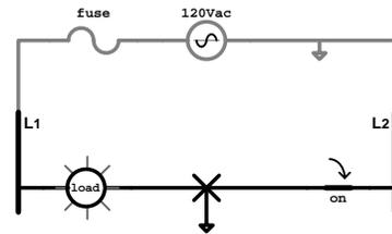
To make matters worse, once the ground fault occurs, the switch is no longer able to de-energize the load! And, if the fault occurs after the load was already energized, there will be no indication of the fault until an attempt is made to shut down the load!
