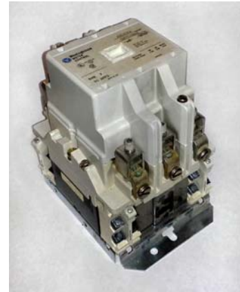
Ratings of Size 3, 90A, 3 \Phi Contactor 200V – 25HP 230V – 30HP 460/575V – 50HP
