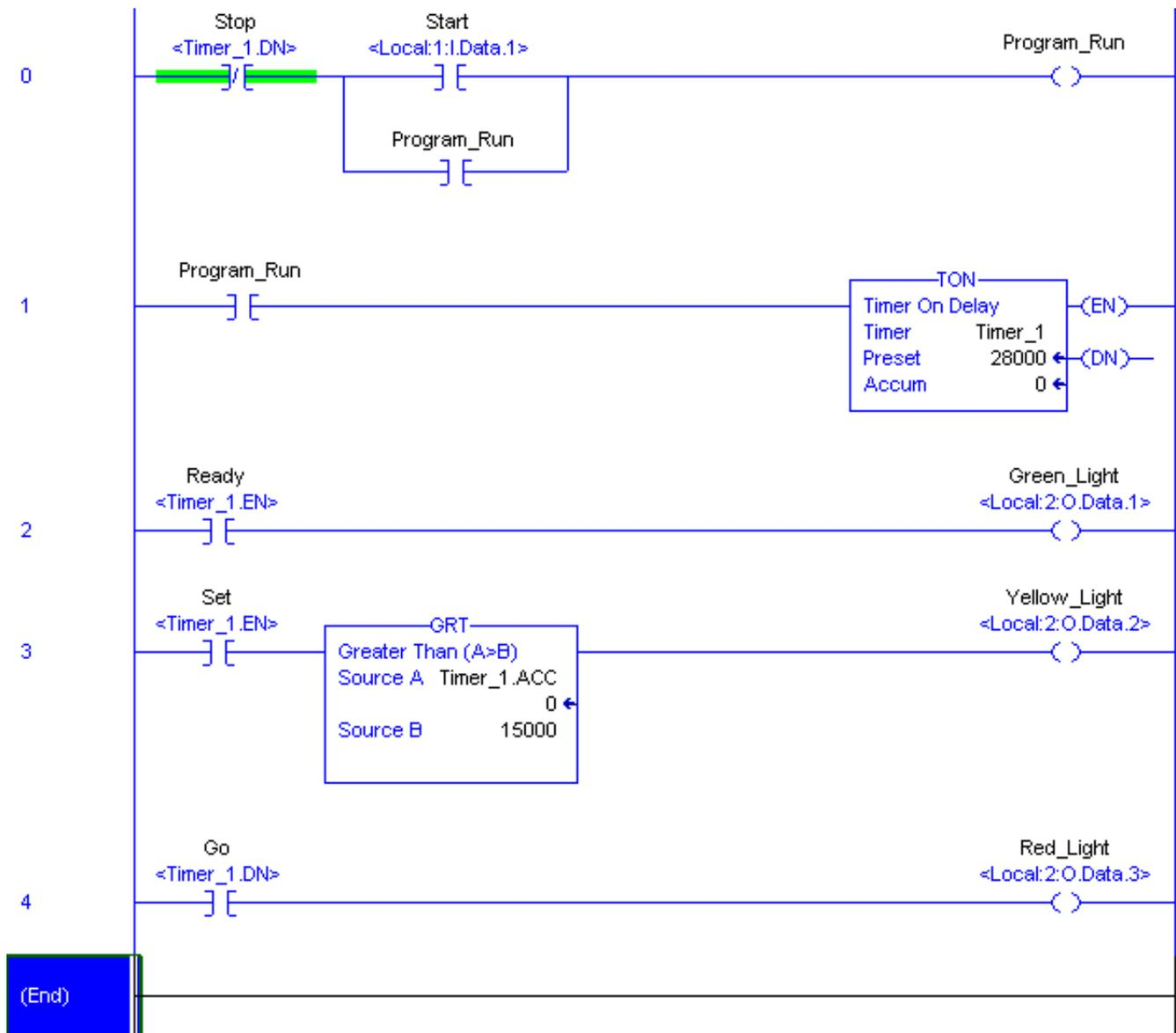
**Figure B – Ladder Logic Diagram #2**
