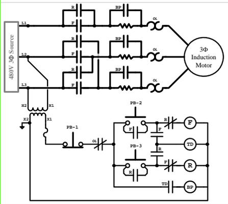
a) Describe in detail the overall motor-control system.
