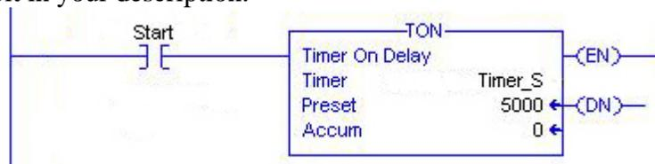
**When the Rung Condition becomes TRUE and remains TRUE for 10 seconds:**
