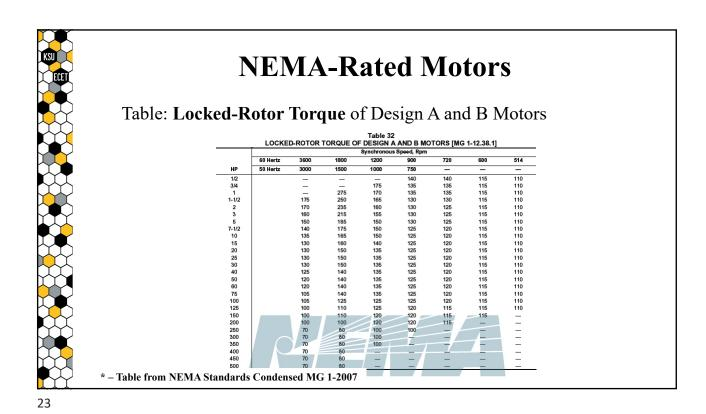
**Locked-Rotor Torque Developed Torque** Locked-Rotor Torque is the amount 300 Design B Breakdown of torque that the motor will develop Torque 250 at standstill when supplied with rated voltage. Breakdown Torque is the maximum instantaneous torque that the motor can develop during normal operation 200 Breakdown Torque is the maximum 150 Locked Rotor Torque 100 without stalling. **Rated Torque** 50 0.9 0.8 -Slip (s) 0.2 0.1 0 Rotor Speed (nr) n Rated Speed 24
