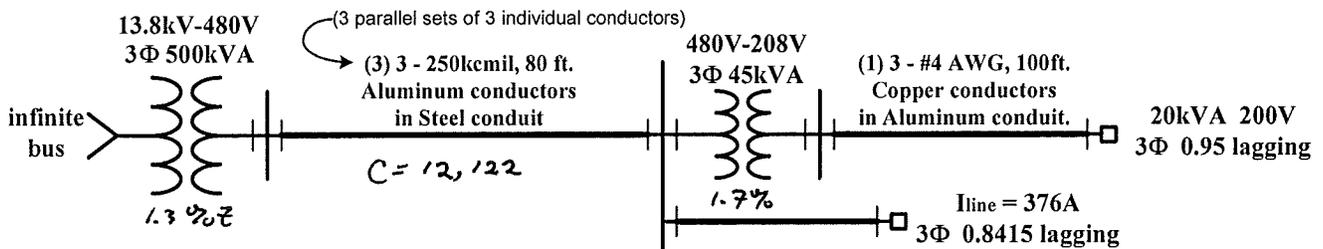
Using the point-to-point method of calculation:
