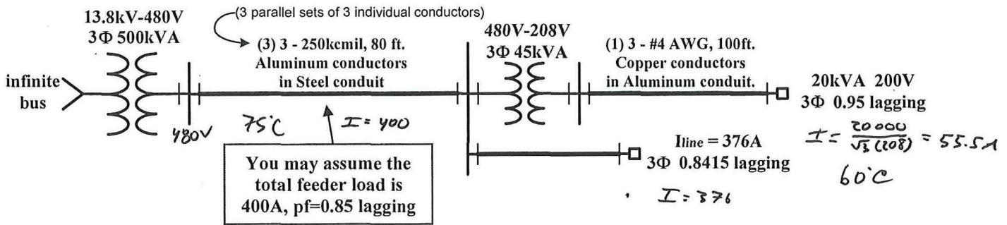
Neglecting any transformer losses, determine the **operational line-voltage** seen at the 20kVA load outlet assuming that rated voltage is present at the secondary terminals of the 500kVA transformer, that the load supplied by the #4 AWG, 100' branch circuit is drawing rated power, and that the total current supplied by the 80' long feeder circuit is 400A at a pf = 0.85 lagging.
