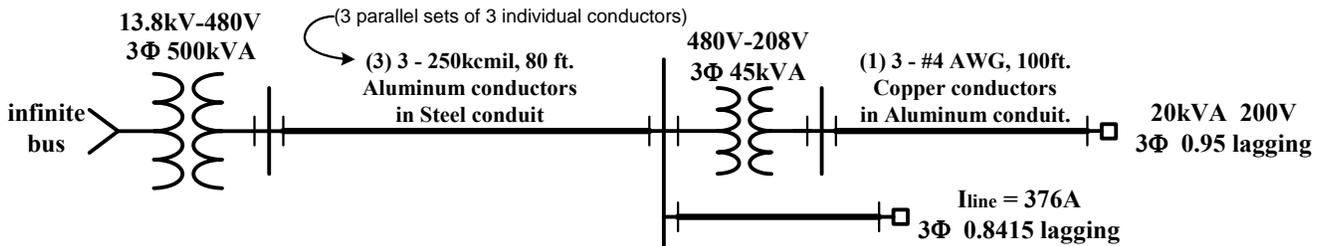
Using the point-to-point method of calculation:
