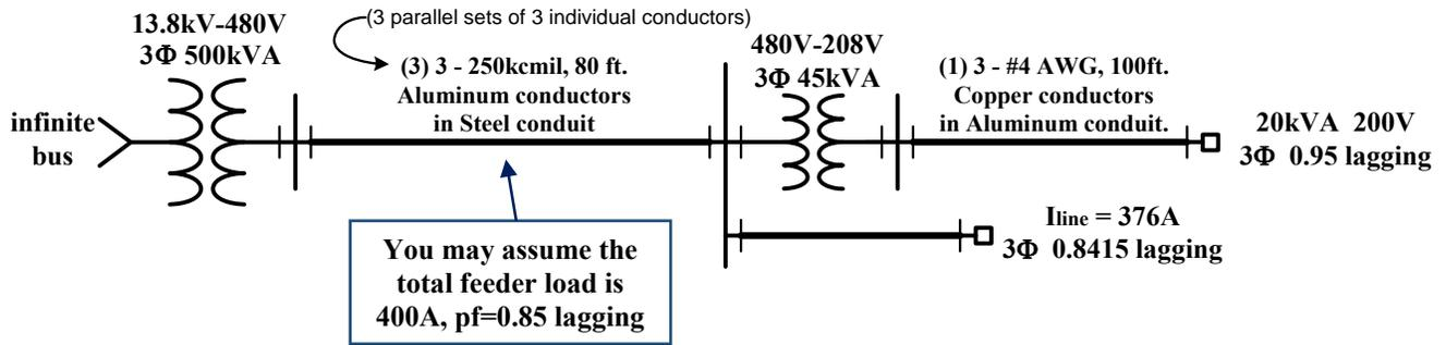
Neglecting any transformer losses, determine the **operational line-voltage** seen at the 20kVA load outlet assuming that rated voltage is present at the secondary terminals of the 500kVA transformer, that the load supplied by the #4 AWG, 100' branch circuit is drawing rated power, and that the total current supplied by the 80' long feeder circuit is 400A at a pf = 0.85 lagging.
