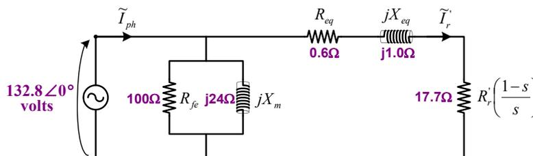
$$V_{ph} = \frac{V_{line}}{\sqrt{3}} = \frac{230}{\sqrt{3}} = 132.8V$$
