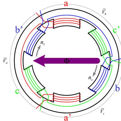
Thus, the three individual (winding) fields combine to form a net “stator field” field that is constant in magnitude but rotates in direction.
