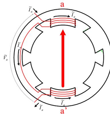
The above figure highlights the phase-A winding, showing the magnetic field that results from a positive winding current. (The “positive” field points from a'→a up through the rotor region).
