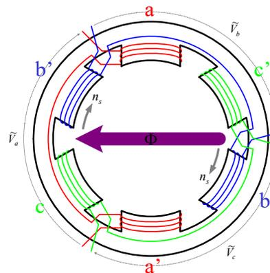
The two-pole stator-field rotates one complete revolution per cycle of the stator excitation.
