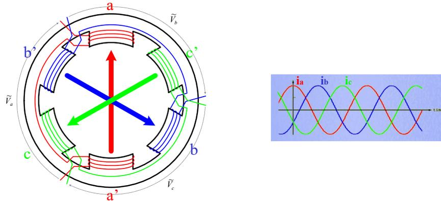
Each winding induces a magnetic field that passes through the machine's "rotor region", the magnitude of which varies proportionally with that winding's instantaneous current.
