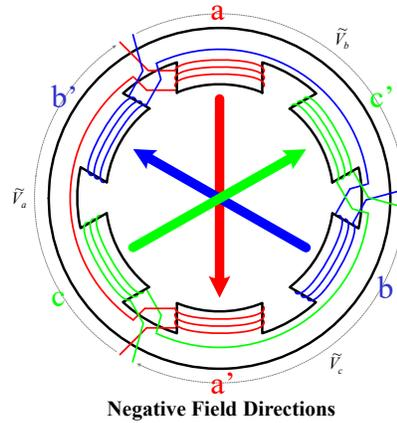
“Negative” instantaneous winding currents result in fields that point in the “negative” directions (as shown in the figure).
