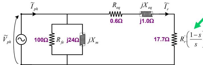
$$n_s = 1200 \text{ rpm} \quad s = \frac{n_s - n_r}{n_s} = \frac{1200 - 1180}{1200} = 0.016\bar{6} \quad \underline{R'_r \left( \frac{1-s}{s} \right) = 0.3 \left( \frac{1 - 0.016\bar{6}}{0.016\bar{6}} \right) = 17.7 \Omega}$$
