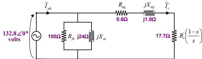
$$\tilde{I}_r' = \frac{\tilde{V}_{ph}}{R_{eq} + jX_{eq} + R_r \left( \frac{1-s}{s} \right)} = \frac{132.8 \angle 0^\circ}{0.6 + j1.0 + 17.7} = 7.246 \angle -3.13^\circ$$
