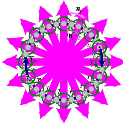
Note that, since the field is constantly rotating, the opposing conductors upon which a torque is developed will vary with the instantaneous position of the stator field.
