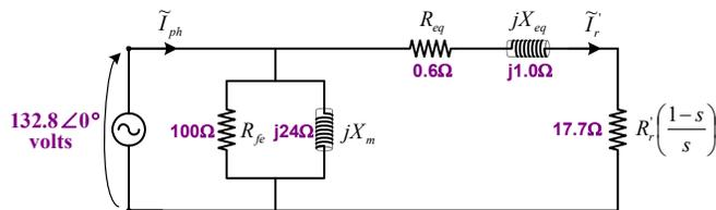
$$P_{shaft} = P_{mech} - P_{mech.losses} = P_{mech} - 190 = 2598 \text{ Watts} = \frac{2598 \text{ Watts}}{746 \frac{\text{Watts}}{\text{hp}}} = 3.482 \text{ hp}$$
