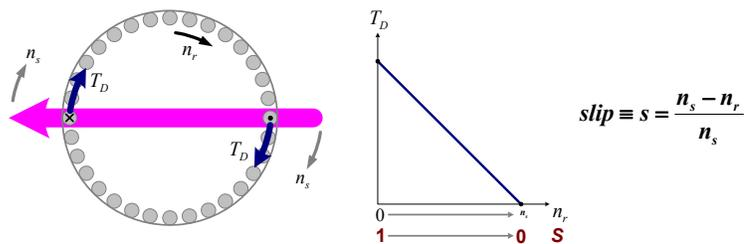
Note – Rotor speed is often expressed in terms of slip, which provides a measure of how much slower the rotor is rotating compared to the speed of the stator field.
