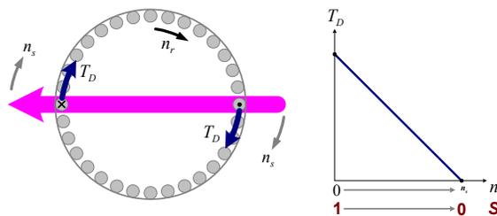
$T_{BR} \equiv$  **Blocked-Rotor Torque**
