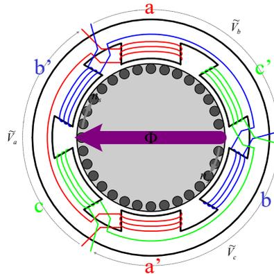
What happens when the squirrel-cage rotor conductors are exposed to the rotating stator field?
