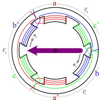
The rotational speed,  $n_s$ , of the "stator field" defines the synchronous speed of the machine... (the speed at which the rotating rotor conductors and the stator field are synchronized).
