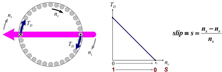
As rotor speed varies from zero to synchronous speed ( $n_r = 0 \rightarrow n_s$ ), the slip decreases linearly from one to zero ( $s = 1 \rightarrow 0$ ).
