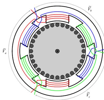
The following presentation covers the construction and operation of a conceptual,  $3\Phi$ , 2-pole, Squirrel-Cage, Induction machine.
