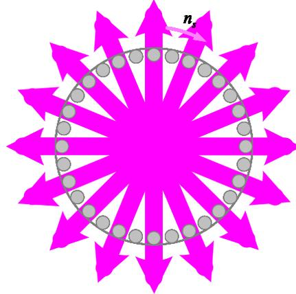
But let's characterize the "stator field" before we investigate the field's interaction with the rotor conductors.
