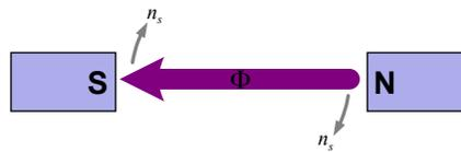
It is called a “two-pole” design because the resultant field is similar to the field that would be created by the opposing poles of two permanent magnets (i.e. – one N pole & one S pole).
