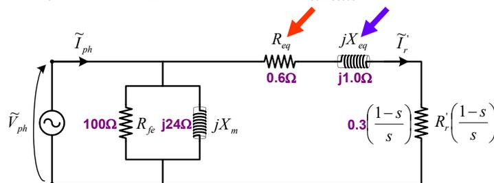
$$\underline{R_{eq} = R_s + R'_r = 0.3 + 0.3 = 0.6 \, \Omega}$$
