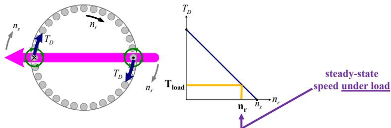
If the rotor is subjected to a load torque after reaching synchronous speed under no-load conditions, then the rotor will slow down to the speed at which the developed torque,  $T_D$ , equals to the load torque,  $T_{Load}$ .
