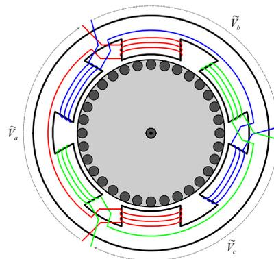
The stator is the stationary (outer) portion of the machine. It provides the primary magnetic field required for operation. This field will be referred to as the “stator field”.
