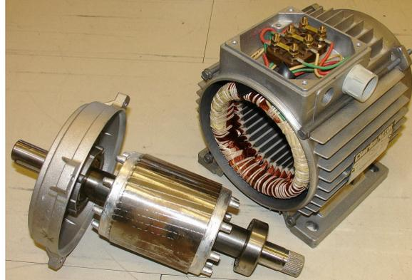
The Three-Phase ( $3\Phi$ ) Induction Machine consists of a stator (stationary portion) and a rotor that are separated by a small air-gap.
