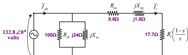
$$S_{source} = 3 \cdot \tilde{V}_{ph} \cdot \tilde{I}_{line}^* = 3 \cdot (132.8 \angle 0^\circ) \cdot (10.4 \angle +34.7^\circ) = 3411 + j2361 = P_{source} + jQ_{source}$$
