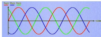
The stator of the machine has three symmetrically-placed windings to which a balanced, 3 $\Phi$  voltage source is connected.
