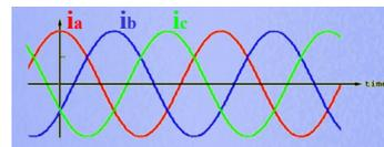
The same principle can be applied to the each of the three symmetrically-placed stator windings in the 3Φ induction machine.
