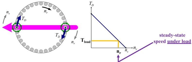
Or, if the rotor is subjected to a load torque at startup, then the rotor will only be able to accelerate up to the speed at which the developed torque,  $T_D$ , equals to the load torque,  $T_{Load}$ .
