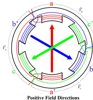
"Positive" instantaneous winding currents result in fields that point in the "positive" directions (as shown in the figure).
