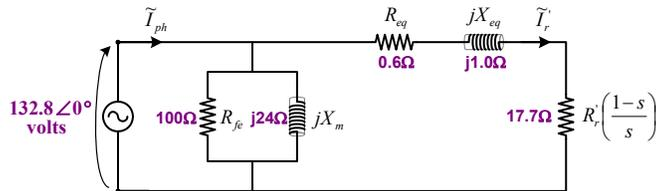
$$Z_{in} = R_{fe} \parallel jX_m \parallel \left( R_{eq} + jX_{eq} + R_r \left( \frac{1-s}{s} \right) \right) = \left( \frac{1}{100} + \frac{1}{j24} + \frac{1}{18.3 + j1.0} \right)^{-1} = 10.4 + j7.26 \Omega$$
