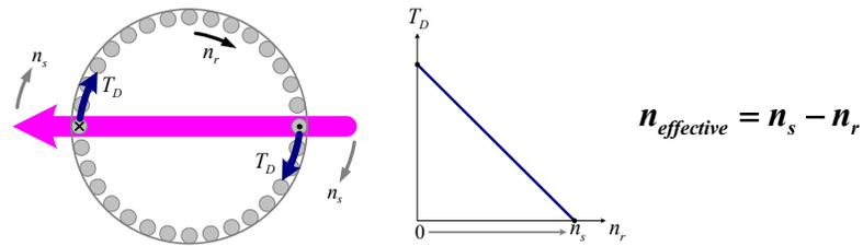
Since the developed torque,  $T_D$ , is proportional to the effective speed,  $n_{effective}$ , at which the stator field cuts across the rotor bars, the developed torque will decrease linearly as the rotor speed increases, eventually decreasing to zero when the rotor is rotating at synchronous speed.
