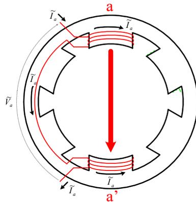
Similarly, the above figure shows the magnetic field that results from a negative phase-A winding current.
