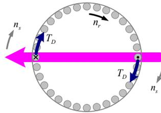
And if there is a positive acceleration torque,  $T_{accel}$ , and the rotor is free to rotate, then the rotor will begin to accelerate the rotor in the same direction as the rotating stator field.
