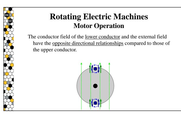
Based upon the <u>field interactions</u>, a **force** will be induced on the <u>upper conductor pointing to the right</u>, while a **force** will be induced on the <u>lower conductor pointing to the left</u>.
