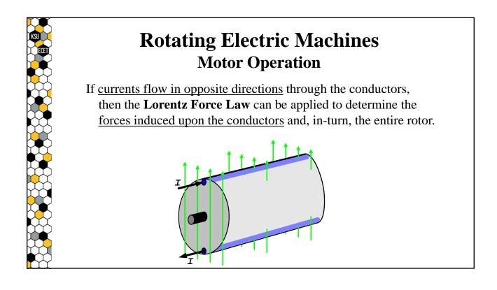
Of key importance is the **direction of the forces** induced upon the conductors. Thus, we will begin by examining the interactions between the <u>conductor fields</u> and the <u>external field</u>.
