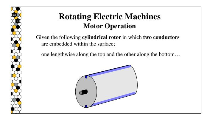
Assume that the rotor is within a region that contains a uniform, **externally-sourced magnetic field**, the lines of which are all vertically oriented through the rotor.
