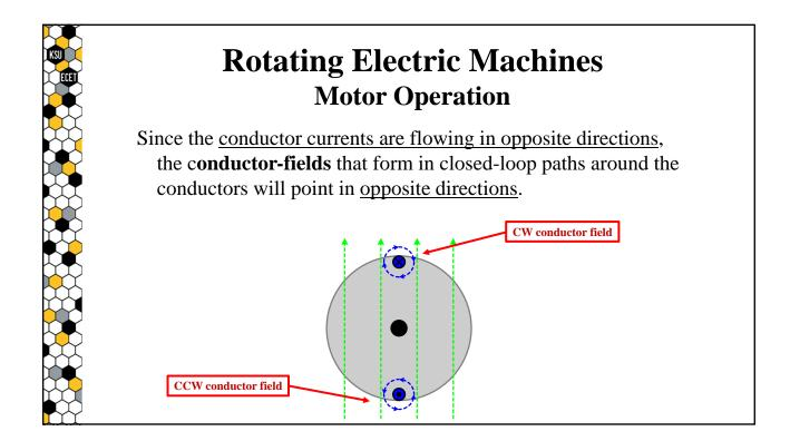
As shown below, the vector-directions of the **conductor field and the external field** are **parallel** in the <u>same direction to the left</u> of the <u>upper conductor</u> and in <u>opposite directions to the right</u>.
