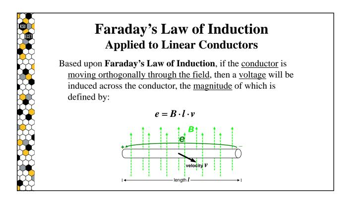
Similarly, if a pair of <u>conductors are embedded within the surface</u> of a rotor that is being <u>rotated</u> by some external means while <u>exposed to a linear external magnetic field</u>...
