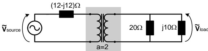
$$\tilde{V}_{\text{load}} = \underline{\hspace{2cm}} \mathbf{62.4 \angle 27.9^\circ} \underline{\hspace{2cm}} \text{ V}$$
