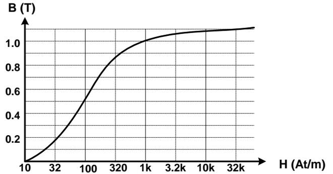
Depends on the exact value of B from plot →  $\Phi = \underline{\quad 34 \times 10^{-6} \quad} \text{Wb}$
