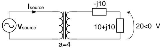
$$V_{\text{source}} = \underline{\hspace{2cm}} \mathbf{56.57 \angle -45^\circ} \underline{\hspace{2cm}} \text{ V}$$
