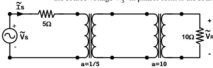
$\tilde{V}_S =$  \_\_\_\_\_  $900\angle 0^\circ$  \_\_\_\_\_  $V$
