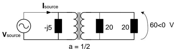
$$\begin{aligned} \tilde{V}_{source} &= \underline{30\angle 0^\circ} \text{ V} \\ \tilde{I}_{source} &= \underline{13.4\angle 26.6^\circ} \text{ A} \\ Z_{inTransformer} &= \underline{2.5+j0} \text{ } \Omega \end{aligned}$$
