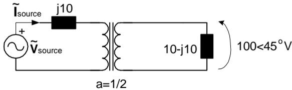
$$\tilde{V}_{\text{source}} = \underline{\hspace{2cm}} \mathbf{111.8 \angle 161.6^\circ} \underline{\hspace{2cm}} \text{ V}$$
