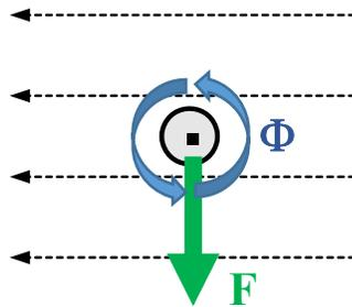
**Problem #20)** Given the system specified in problem 19, if the flux density of the external field is **0.5 Tesla** and the conductor has an effective length of **4 meters**, determine the **current** required in the conductor to create a force of **3.2 N** on the conductor, along with the **voltage induced** on the conductor if it is traveling orthogonally through the field at a velocity of **17.8 m/sec**.
