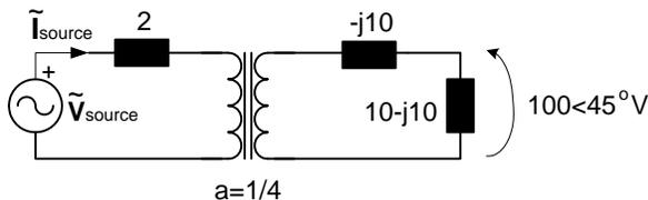
$\tilde{V}_{source} = \underline{\quad 82.23 \angle 64.54^\circ \quad} \text{V}$
