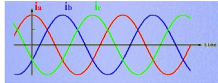
The stator of the machine has three symmetrically-placed windings through which a balanced set of 3 $\Phi$  currents will flow when supplied by a balanced, 3 $\Phi$  voltage source.
