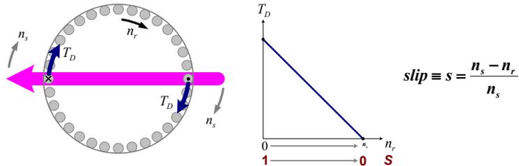
**Note – Rotor speed is often expressed in terms of slip, which provides a measure of how much slower the rotor is rotating compared to the speed of the stator field.**
