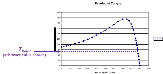
In terms of torque, rated load ( $T_{rated}$ ) for an induction motor is the maximum steady-state torque that the motor can develop without overheating while supplied at rated voltage.
