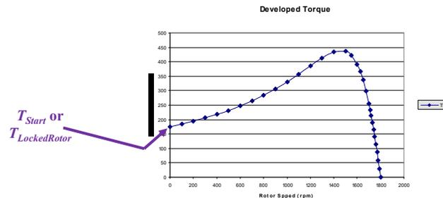
Note that at startup or under “locked-rotor” conditions, the motor will draw a line current that is much larger than the motor’s rated current, typically 4-10x larger.
