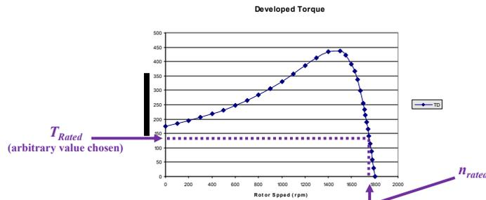
The speed the motor operates at while driving rated load is defined as the motor's rated speed ( $n_{rated}$ ).
