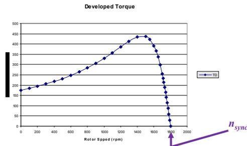
Similar to an “ideal” machine, a practical machine will still accelerate to its synchronous speed and run steady-state at that speed while under ideal “no-load” conditions.
