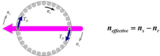
Note that the developed torque,  $T_D$ , is proportional to the rate at which the stator field cuts across the rotor conductors.
