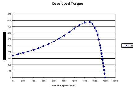
The torque-speed curve for a practical 4-pole, 60Hz induction machine is shown above.
