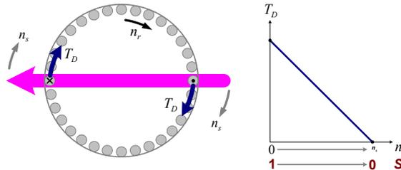
$T_{BR} \equiv$  **Blocked-Rotor Torque**
