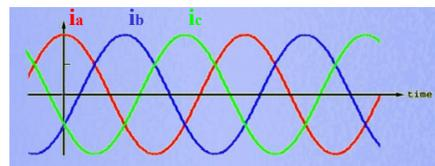
Each winding current induces an instantaneous magnetic field, the vector sum of which results in a net magnetic field that passes linearly through the “rotor region”.
