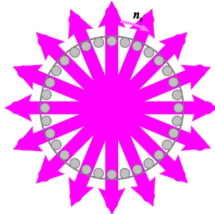
And, since the “stator field” passes through the rotor region, the squirrel-cage rotor conductors will be exposed to a time-varying (rotational) magnetic field.
