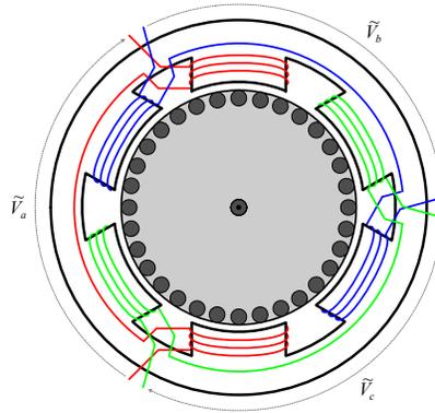
The rotor is the rotational portion of the machine that provides the mechanism for energy conversion (elec→mech or mech→elec) as it interacts with the stator field.
