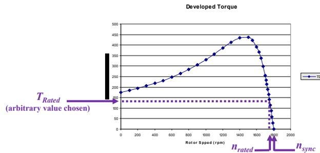
Normal operation for the motor can be defined as operation of the motor while supplied at rated voltage and driving no more than rated load. ( $0 \leq T_D \leq T_{Rated}$ )
