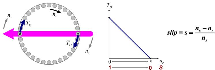
**As rotor speed varies from zero to synchronous speed ( $n_r = 0 \rightarrow n_s$ ), the slip decreases linearly from one to zero ( $s = 1 \rightarrow 0$ ).**
