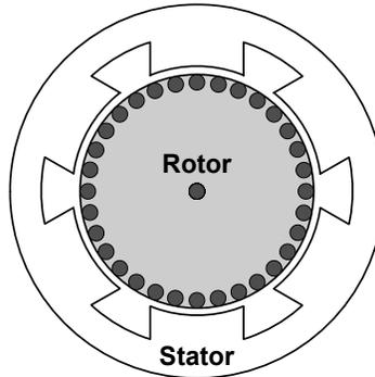
A “Squirrel-Cage” rotor is constructed as a cylinder with a set of conductive bars embedded just under its surface, allowing for only a small air-gap between the rotor and the stator.
