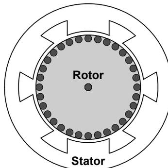
The ends of the conductive bars are shorted together by a pair of conductive rings, forming the “Squirrel-Cage” aspect of the rotor and providing closed-loop paths for currents to flow.
