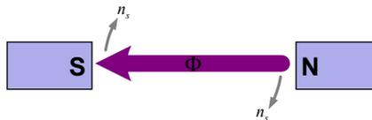
It is called a “two-pole” design because the resultant field is similar to the field that would be created by the opposing poles of two permanent magnets (i.e. – one N pole & one S pole).
