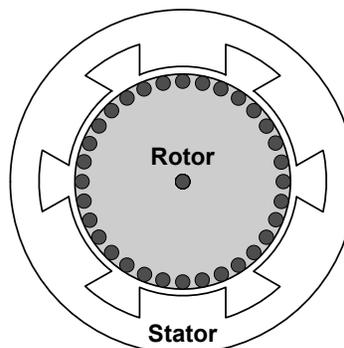
The construction of the rotor determines the type of induction machine. As stated, this presentation will focus on the Squirrel-Cage type of rotor construction.
