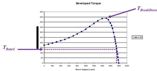
The **breakdown torque** ( $T_{BreakDown}$ ) for the machine is defined as the maximum torque that the motor is able to develop after it is already running under normal operating conditions.
