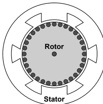
**Note – The rotor itself is constructed using laminated sheets of steel. The laminations provide insulation between the sheets, preventing currents from flowing length-wise through the rotor unless they actually travel through the embedded conductive bars.**
