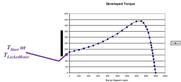
At startup or under “locked-rotor” conditions ( $n_r = 0$ ), the motor is only able to produce a limited amount of torque.
