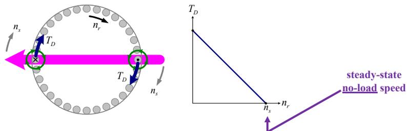
The torque-speed curve for an “ideal” induction machine is shown above for rotor speeds ranging from zero  $\rightarrow$   $n_s$ .
