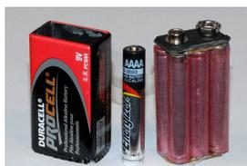
Internally, a 9V battery contains **six** individual **cells**, each the size of a AAAA battery, that are wired together to produce a total of 9V.
