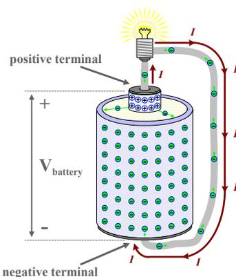
The **terminals** of the battery provide an external connection to its charged regions in order to allow for the **developed voltage** to be used as a source of **current** that will flow out of the positive terminal, through an externally-connected electric circuit, and back into the negative terminal.
