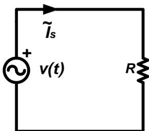
$v(t) = \sqrt{2} \cdot 120 \cdot \sin(\omega \cdot t + 20^\circ)$  volts     $f = 60 \text{ Hz}$
