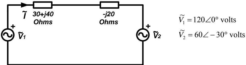
Write out the Kirchhoff's Voltage Law (KVL) equation that could be used to solve the current  $\tilde{I}$ , expressing the voltages across the impedances based on the direction of the current  $\tilde{I}$  as shown, and use the equation to determine the phasor current  $\tilde{I}$ .
