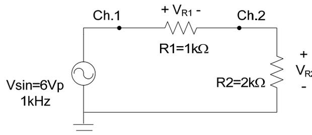
**Figure 8.2: AC Series Circuit.**
