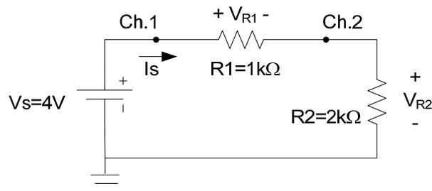
**Figure 8.1: DC Series Circuit.**
