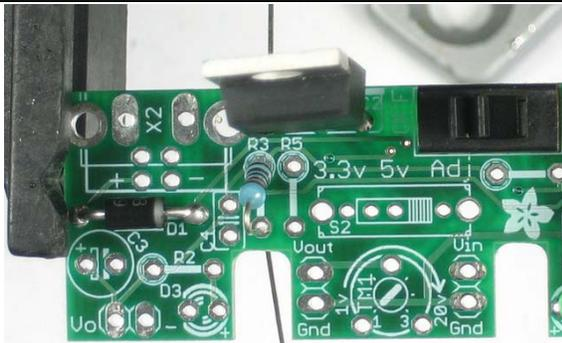
The regulator uses resistors to set the adjustable output voltages. We'll now solder those in.
