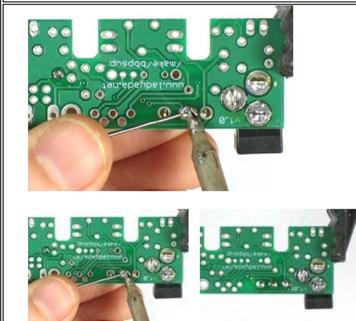
Tape or hold the switch in place while you solder all three pins.
