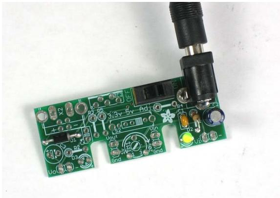
Lets take a break and test the current progress. Take the kit out of the vise and make sure there are no stray wires kicking around that could cause the board to short.
