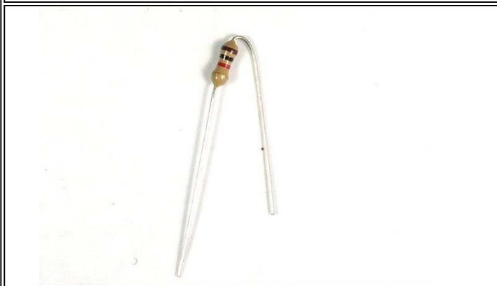
We're going to solder one of the 1.0K resistors in next. The resistors should be bent over 180 like shown. Note that resistors are 'non-polarized' so you can put them in 'either way' - they work the same forwards or backwards.
