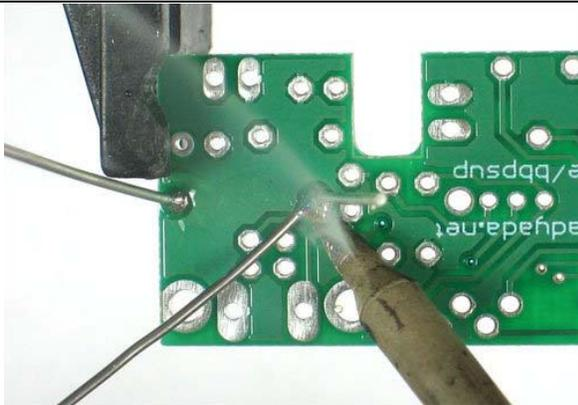
Now solder both wires to the PCB.
