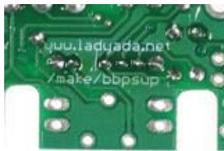
Be careful because the solder points are small and somewhat close together. Make sure you don't have a short circuit and that each point is soldered.
