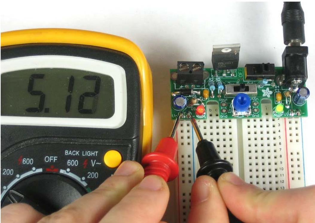
Finally, by selecting **Adj.** you can adjust the supply to anything you want from as low as  $\sim 1.3\text{V}$  to within half a volt of the input (which can be as high as 20V).
