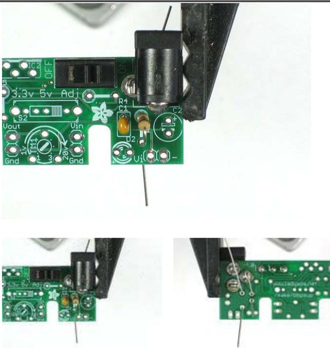
Place one of the 1.0K resistors (Brown Black Red Gold) into the slot marked R1. Then place right next to it one of the 0.1uF ceramic capacitors (they're small and yellow). The resistors and ceramic capacitors are non-polarized so they can go in 'either way'.
