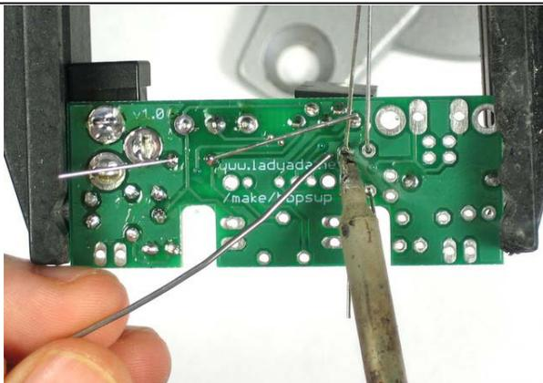
Solder and clip the three resistors.
