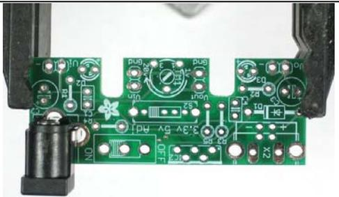
We'll start by placing the DC power jack. This is how we will attach outlet power supplies to the board. The jack is 2.1mm which is the most common size.
