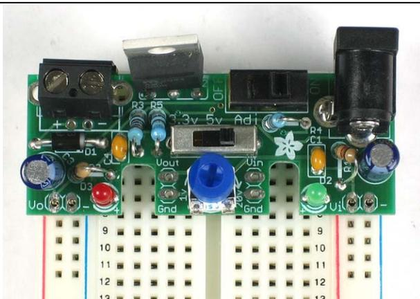
Now place the power supply on top. If it fits nicely, solder the four pins.
