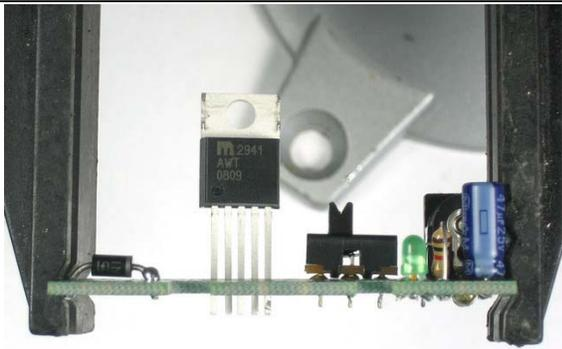
Now we will solder in the heart of the kit, the MIC2941 adjustable voltage regulator. The regulator must be placed correctly to work. Make sure that the big silver tab is at the edge of the PCB (there is a thick white line on the silkscreen to indicate it).
